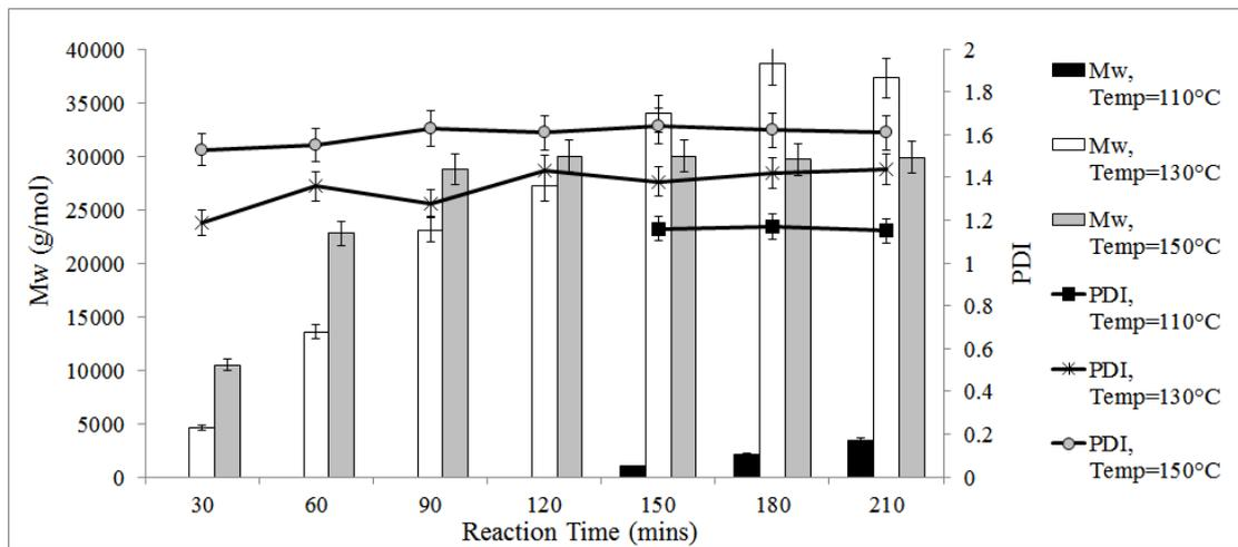
**Figure 3.6:** Mw and PDI at various reaction temperatures ( $\text{Sn}(\text{Oct})_2$  concentration kept at 0.00868 mol/L and benzyl alcohol concentration kept at 0.01159 mol/L)
