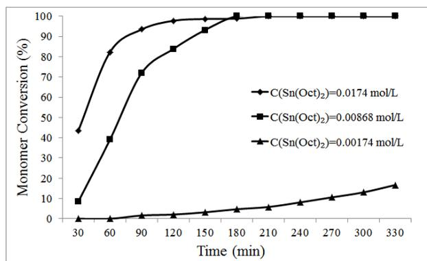
**Figure 3.1:** Monomer conversion rate at various  $\text{Sn}(\text{Oct})_2$  concentrations (Benzyl alcohol concentration kept at 0.01159 mol/L and the polymerisation temperature kept at 130°C)
