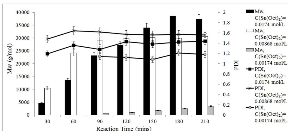
**Figure 3.2:** Mw and PDI at various  $\text{Sn}(\text{Oct})_2$  concentrations (Benzyl alcohol concentration kept at 0.01159 mol/L and the polymerisation temperature kept at 130°C)
