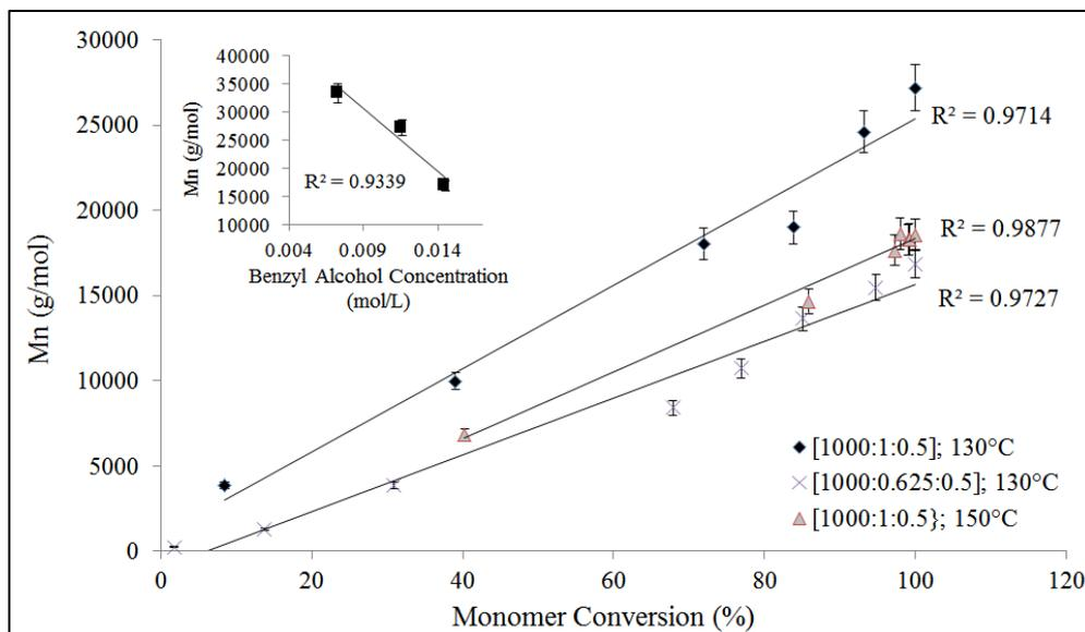
**Figure 3.7:** Mn against monomer conversion rate with different reaction parameters (Inner figure shows Mn against initiator Benzyl alcohol concentration variation,  $\text{Sn}(\text{Oct})_2$  concentration and reaction temperature kept at constant)
