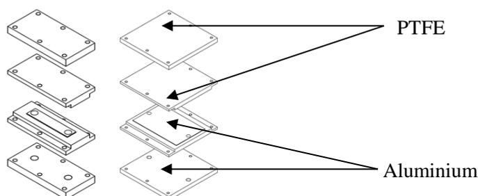
**Figure 2.2:** PTFE moulds for ISP
