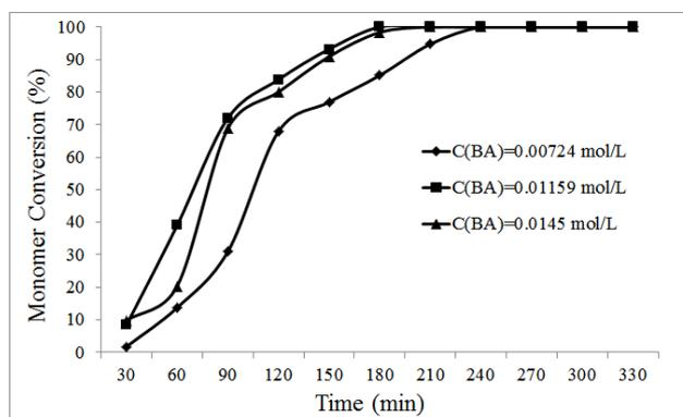
**Figure 3.3:** Monomer conversion at various benzyl alcohol concentrations ( $\text{Sn}(\text{Oct})_2$  concentration kept at 0.00868 mol/L and the polymerisation temperature kept at 130 °C)
