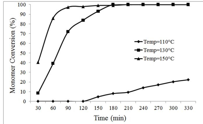
**Figure 3.5:** Monomer conversion at various reaction temperatures ( $\text{Sn}(\text{Oct})_2$  concentration kept at 0.00868 mol/L and benzyl alcohol concentration kept at 0.01159 mol/L)
