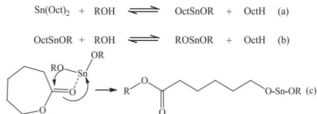
**Figure 2.1:** Initiation and propagation reactions for CIM polymerisation of  $\epsilon$ -caprolactone
