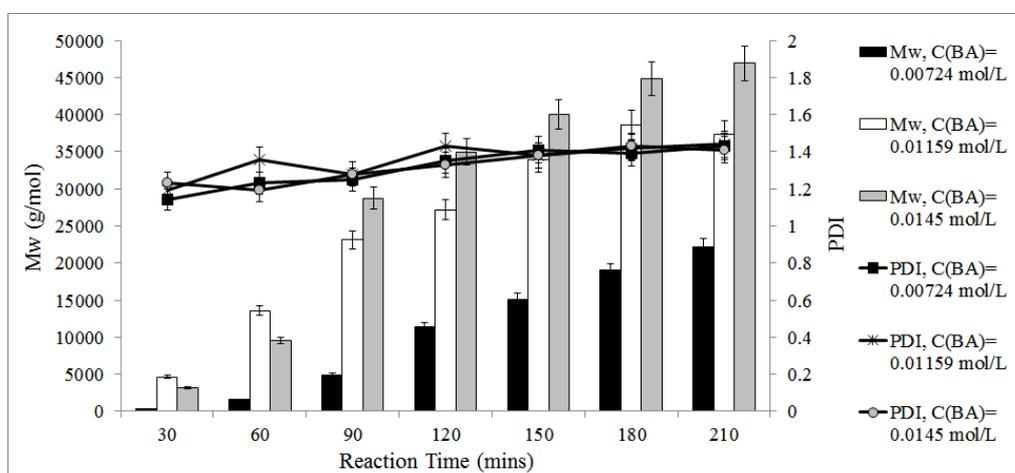
**Figure 3.4:** Mw and PDI at various Benzyl alcohol (BA) concentrations ( $\text{Sn}(\text{Oct})_2$  concentration kept at 0.00868 mol/L and the polymerisation temperature kept at 130 °C)
