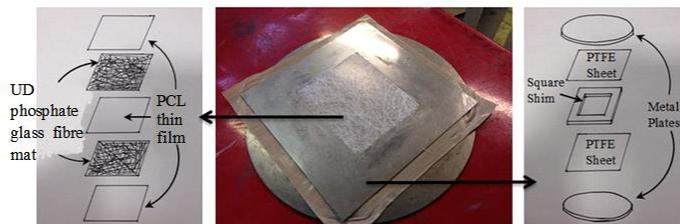
**Figure 2.3:** Film stacking assembly for hot press moulding
