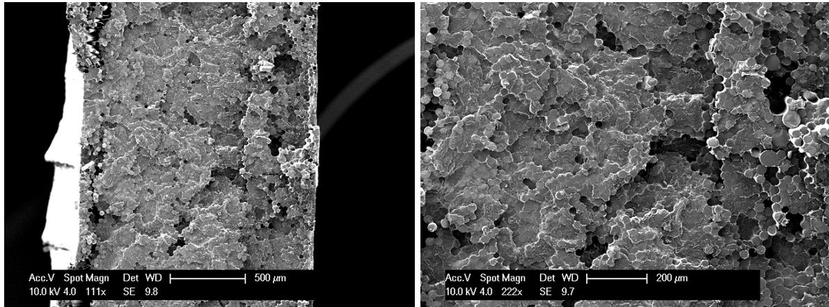
**Figure 3.9:** SEM images of fractured surfaces of the ISP35 UD composites manufactured via ISP
