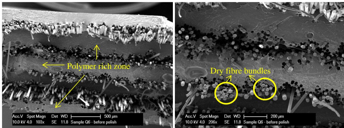
**Figure 3.8:** SEM images of fractured surfaces of the LS35 UD composites manufactured via LS
