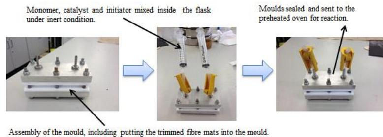
**Figure 2.4:** ISP composites production procedures
