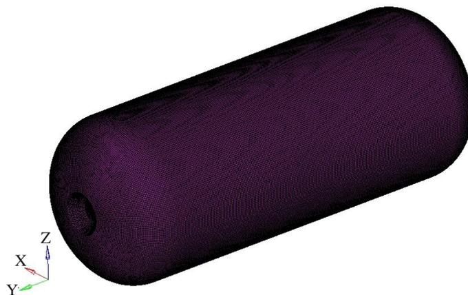
Figure 3: Mesh of liner.
