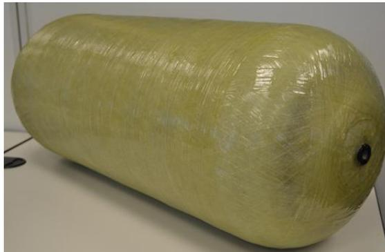
Figure 1: Type IV CNG tank.
