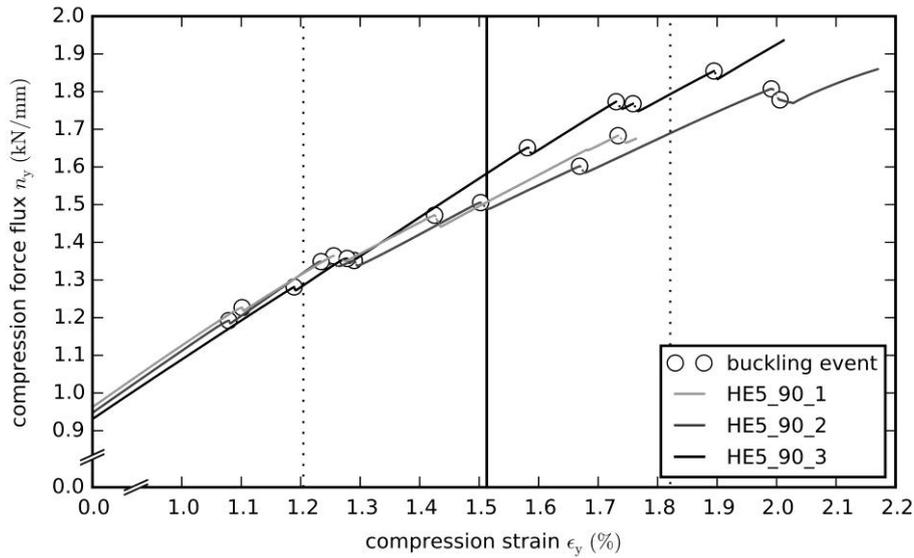
Figure 6: Strain gauge compressive strain against line load of 3 samples. Buckling of a bundle is indicated by a circle. The end of the load/strain curves represents final failure. The experimental mean buckling strain with Gaussian standard deviation (17 events) of  $1.513 \pm 0.308$  % is plotted.
