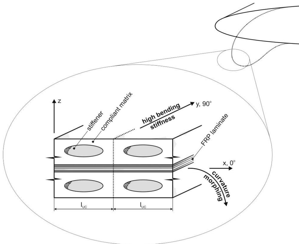
Figure 1: Sketch of the structural concept of the leading edge skin.
