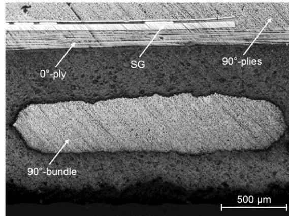
Figure 3: Microscope image of a polished section taken with a Zeiss Axio Lab.A1 (5x object lens). A complete rubber embedded bundle together with the location of the strain gauge is visible.
