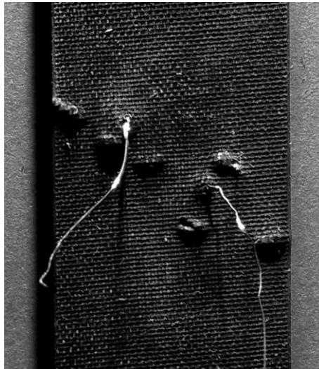
Figure 7: Photography of the section between the supports of a sample after testing. All 6 bundles of the hybrid layer have been irreversibly buckled.
