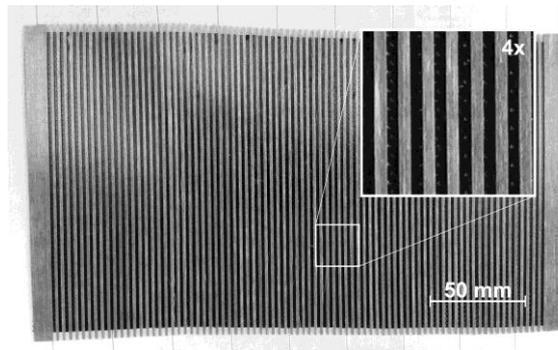
Figure 2: Stacking process step at which the cut bundles are placed above a rubber ply (black background).
