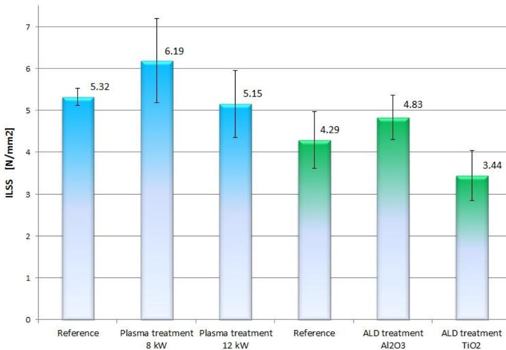
Figure 6: The ILSS results for the plasma and ALD treated samples and corresponding untreated reference samples.
