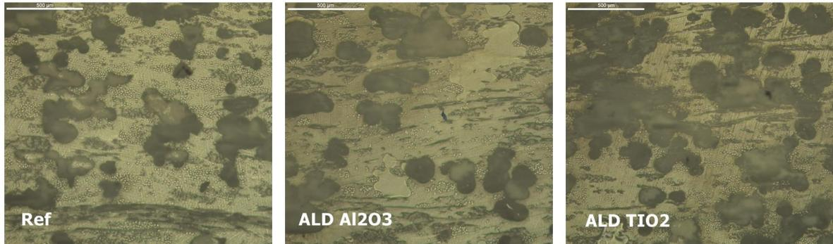
Figure 8: Microscope pictures of ALD treated samples and reference. Scale bar is 500 µm
