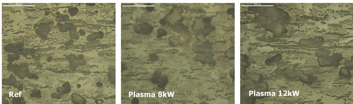
Figure 7: Microscope pictures of plasma treated samples and reference. Scale bar is 500 μm
