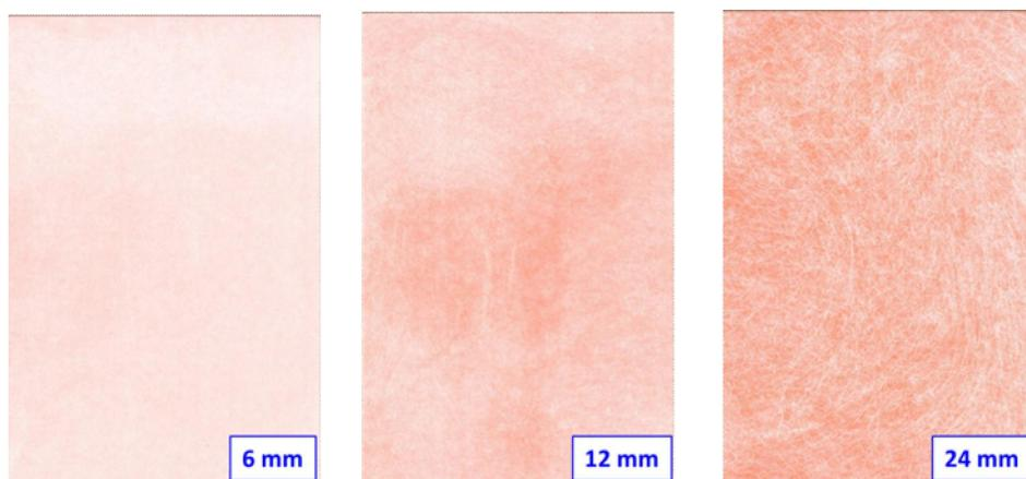
Figure 1: Foam-formed laboratory sheets obtained with viscose fibres. The homogeneity of the structure is preserved for the varied fibre lengths (6, 12 and 24 mm).
