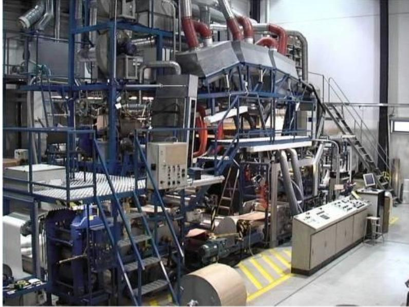
Figure 2: Extrusion coating and lamination pilot line at Tampere University of Technology. Maximum line speed at the pilot line is ~ 400 m/min and maximum web width 550 mm.
