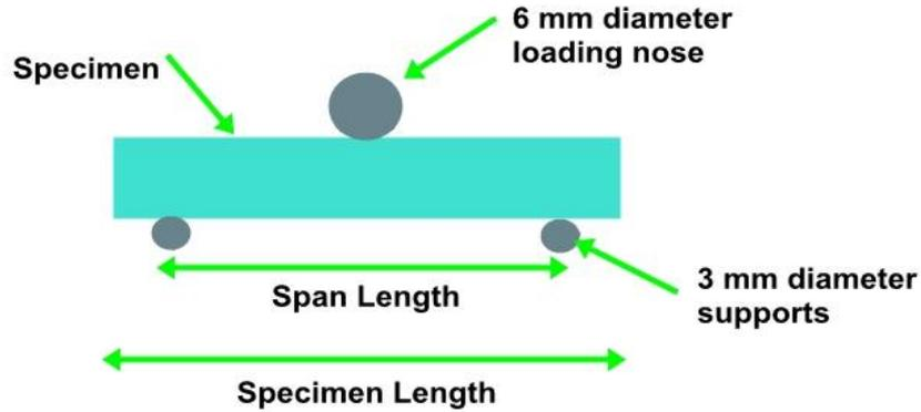
Figure 5: ILSS test configuration
