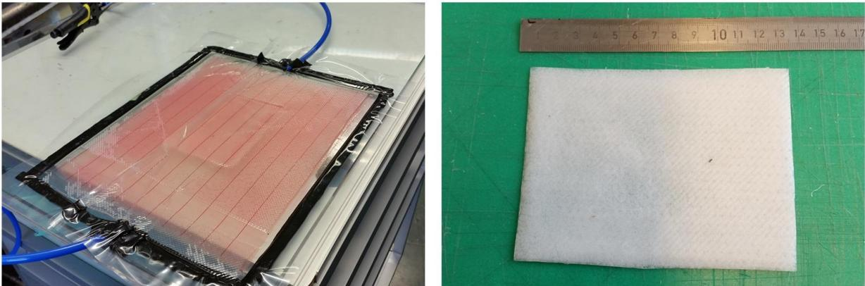
Figure 4: On the left vacuum assisted resin infusion of the sample. On the right is ready laminate sample 13 x 10 cm.
